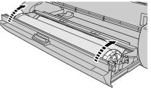
**4** Remove the roll holder, remove the holder stopper, then remove the media.
